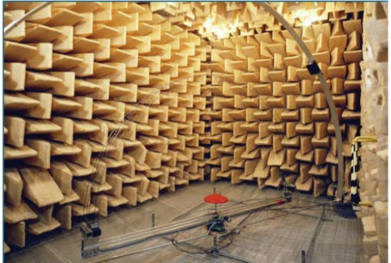
Figure 1. Left: 2D boundary plane goniometer; Right: 3D goniometer in an anechoic chamber
