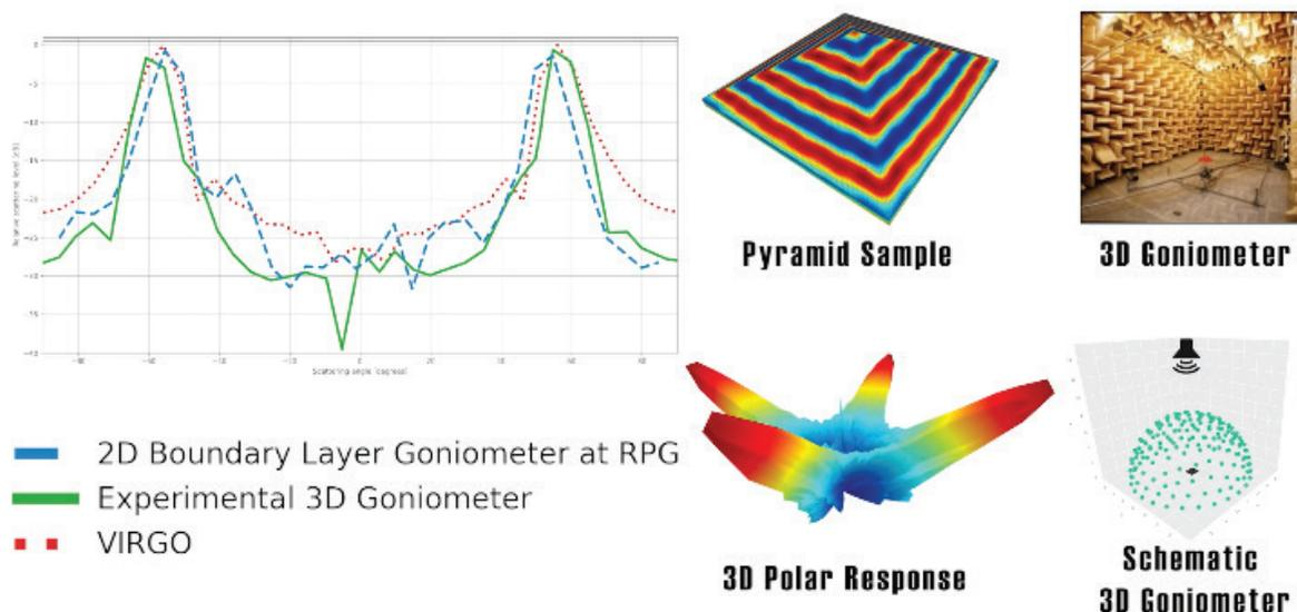
Figure 3. Comparison between the 2D and 3D goniometer normal incidence 2 kHz polar responses measured according to ISO 17497-2 and the simulated response from Virgo.
