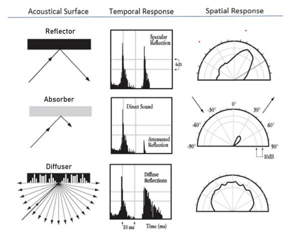
The Temporal Response of the Reflector is a slightly attenuated and delayed version of the direct sound, the Absorber significantly attenuates the direct sound, and the Diffuser provides a dense array of diffuse reflections covering a time related to the depth of the unit, with roughly the same energy as the direct sound.
